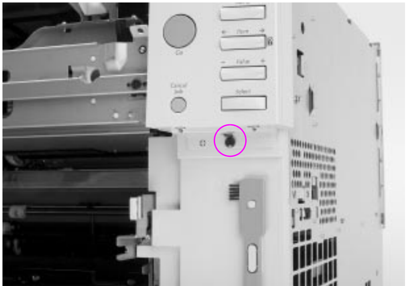
Figure 6-11 Control panel removal and replacement
